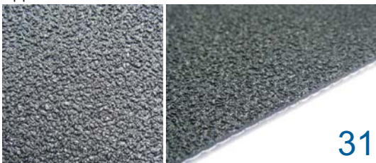
Name:Sandblast Thickness:0.2mm Property:Non adhesive surface,medium friction Application:Logistic,Treadmill belt, Roller wrapping
